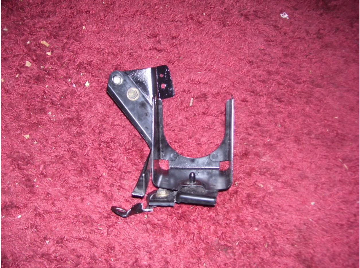
Modified abs bracket so it will fit near battery tray.
