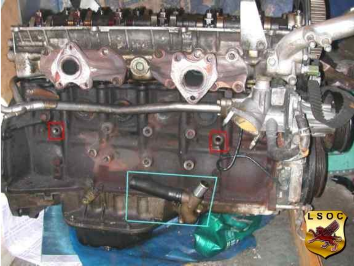
Remove the oil return flange shown below. Undo the 2 bolts marked in RED.
