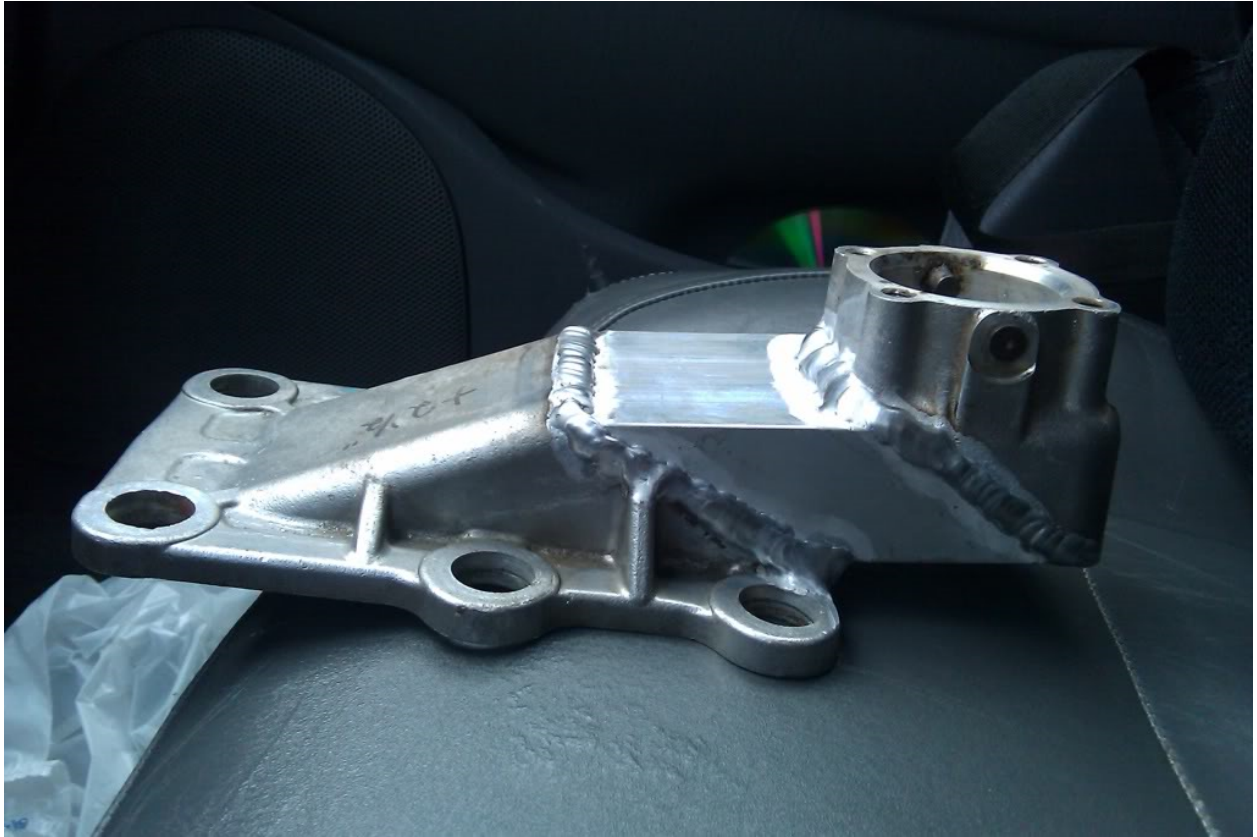
Shifter Extension for R154 (Requires use of a straight shifter)
